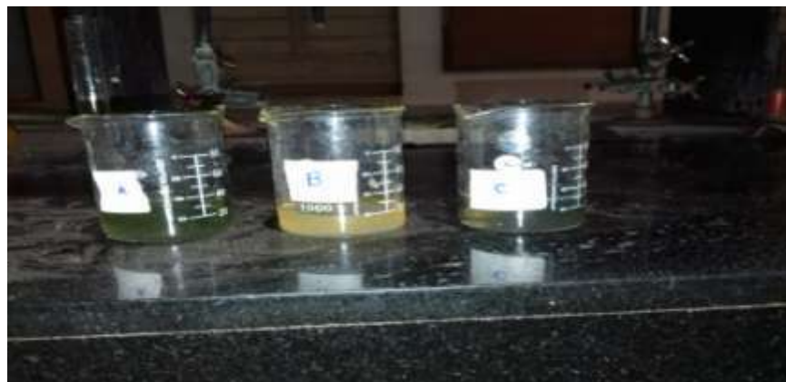
Figure 1: Visual observations of A - Leaf extract, B - Ferric chloride, C - Iron oxide Nanoparticles
