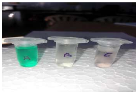
Figure 1. Synthesis of nickel nanoparticle A-Std Ni solution, B- Leaf extract, C- Ni solution + Leaf extract
