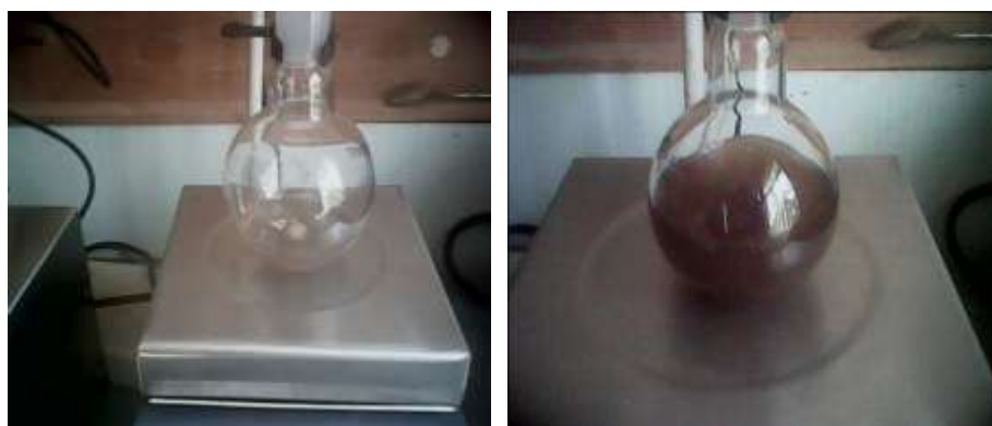
Fig. 2 a) Solution of silver nitrate 1 mM before. b) Reddish brown colour formed due to reduction.
