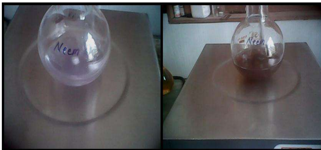
Figure 1: Solution of silver nitrate 1mmol L -1 before (left) and after (right) addition of Azadirachta indica leaf extracts solution
